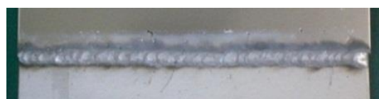
(a) MIG溶接
